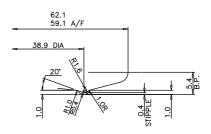
STACKING RING DETAIL - SCALE 3:1
